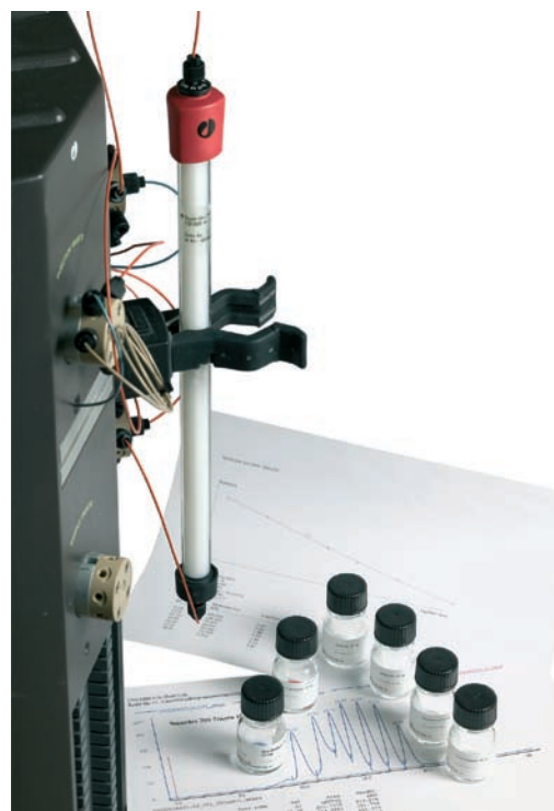
Fig 1. Gel Filtration Calibration Kit LMW and HMW are two kits for calibration of gel filtration columns.
