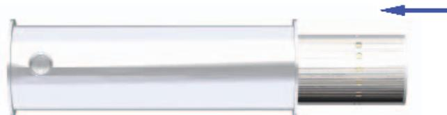
3. Slide membrane filter cartridge (which now has one O-ring in position) into one end of housing. Clamp end cap.
